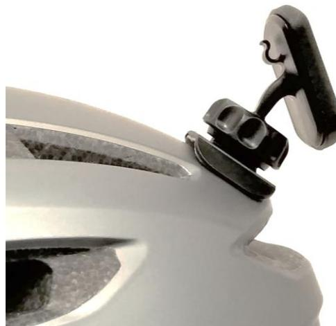
**Step 8.** Attach the ListenTALK transceiver leader unit via the magnetic pad on the SCOSCHE mount as shown below. With the front of the unit positioned facing back towards the participants, securely tighten the adjustment knob on the SCOSCHE mount. Attach desired leader headset/mic. The unit can be easily removed from the magnetic pad for configuration or charging in the ListenTALK charging dock, when needed.
