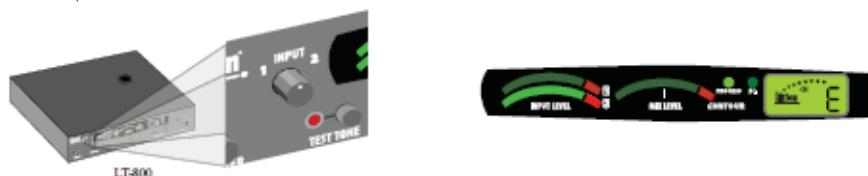
3. Now with the microphone turned Off or not active, adjust the music player's volume so that the level on the left "Input Levels" meter is hitting 1/2 to 3/4 of the green LED's (No red LED's).
