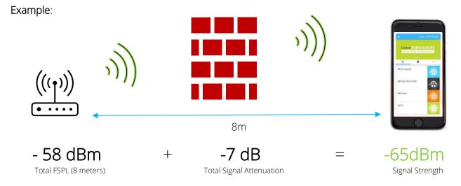
After calculating the signal strength, one can determine a fairly accurate measurement of the signal quality with the chart below. It is strongly advised that there should be no less than - **70dBm while using the Listen Everywhere system**. This ensures that the UDP packets are delivered more quickly and more reliably.
