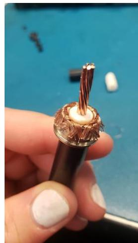
10. The inner copper conductor is made up of seven strands of solid copper wire. Pull back three of those strands in a circular pattern as shown to the right
