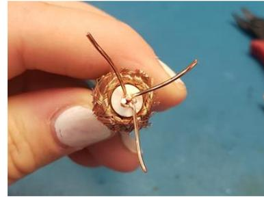
11. Cut those three strands as close to the edge of the inner white plastic as shown. If they are not cut properly then they could cause the cable to fail.
