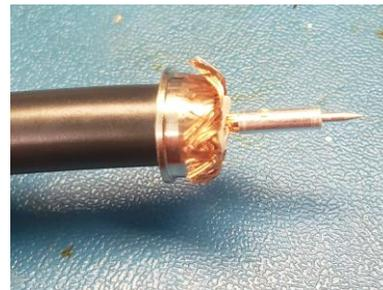
13. Place the cable into the table vice. Remove the center pin and apply some flux and tin the copper conductor sparingly. The fit inside the center pin can be very snug. Too much solder can make it difficult to place the center pin over the copper conductor again.
