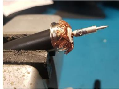
15. Now use the outer BNC connector from the LA-128 package and slide it over the center pin and cable, ensuring the center pin's tip does not extend beyond the end of the BNC connector. You want to be able to feel the tip when you press it with your finger, but you do not want it to stick far enough out that it can be blunted and damaged with use.
