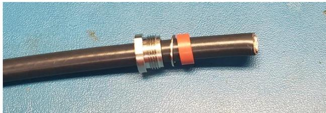
4. Measure 1/2" from the end of the cable and strip the outer black plastic covering as shown below. (Do not damage the copper braid as seen below).
