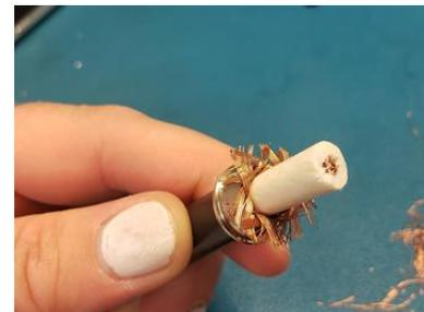
8. Trim the end of the cable so that it is not longer than  $\frac{1}{2}$  inch from the top of the angled washer and copper braid.
