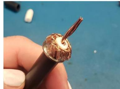
12. On the four additional inner copper conductors, spin them together tightly using the pliers as shown. Make sure the length of the inner copper conductor fits snugly inside the center pin and is seated as far down as possible. There should only be a little bit of the inner copper conductor visible between the bottom of the pin and the top of the white insulation.
