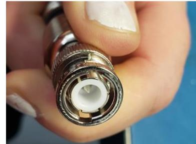
16. Slide the rubber washer, metal washer and threaded cylinder back up the cable and into the outer BNC connector.
