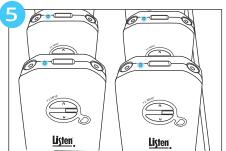
LED status: flashing- charging, solid- fully charged
