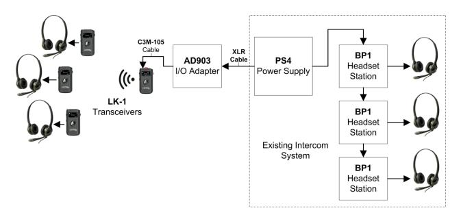
Note: The Pro Intercom C3M-105 cable <u>must</u> be used to interconnect the LK-1 Leader unit and the AD903 adapter. An XLR cable is needed to interface the AD903 with the existing intercom's power supply.
