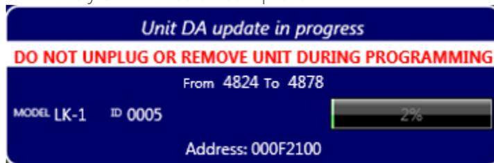
9. After the DA update has been completed, the red slash symbol will no longer appear on the unit. Select the unit and click the info button to verify the Update DA button is no longer red and the Current Version and Pair Version match.
