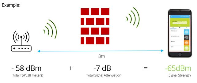
After calculating the signal strength, one can determine a fairly accurate measurement of the signal quality with the chart below. It is strongly advised that there should be no less than - 70dBm while using the Listen Everywhere system. This ensures that the UDP packets are delivered more quickly and more reliably.
