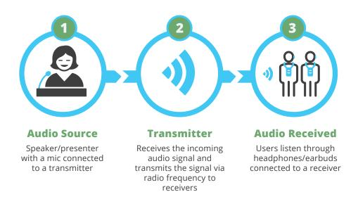
Listen Technologies is the only manufacturer that offers systems that operate in 216 MHz frequency range. This allows the user to move around in large venues without losing the signal. This also simplifies the distribution of receivers as they all work in the same frequency and don't need to be coordinated or based on where an individual is seated.
