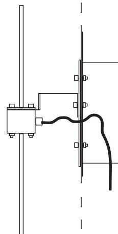
Diagram B. The Electrical Box Mount uses the Mounting Plate and Mounting Bracket as shown above.
