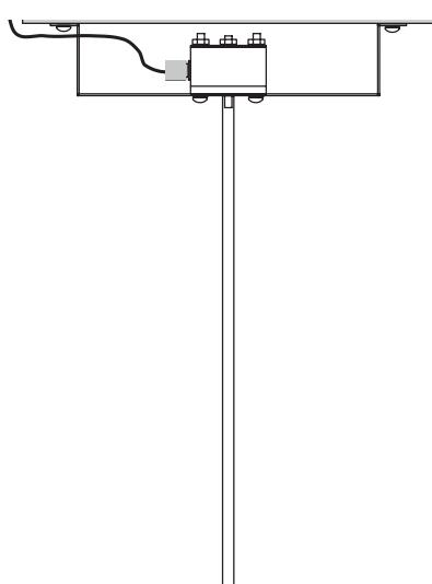
Diagram K. Inverse Mounting of a monopole.
