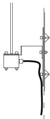
Diagram C. A direct Wall Mount should use the Mounting Plate for added strength, but it is not required for proper antenna operation.
