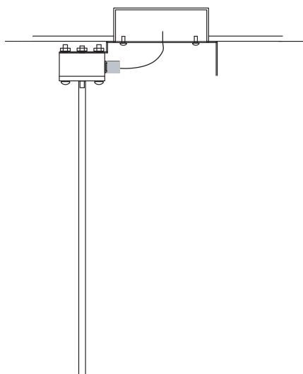
Diagram H. Ceiling mounted monopole with a grounded box.
