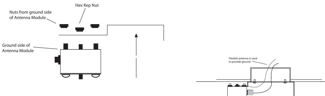
Diagram G. Reversing the antenna Module on the Mounting Bracket.
