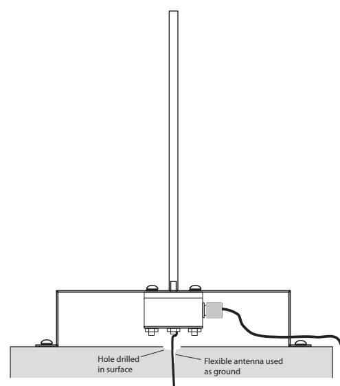
Diagram L. Mounting a monopole on a non-conductive surface. Use of the flexible wire creates a dipole, which is a better antenna than the monopole.
