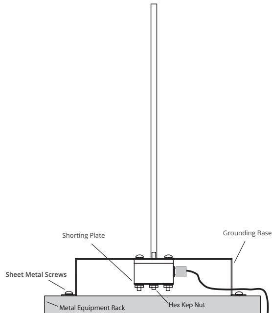
Diagram J. A reversed Antenna Module with Ground Plane and Shorting Plate.
