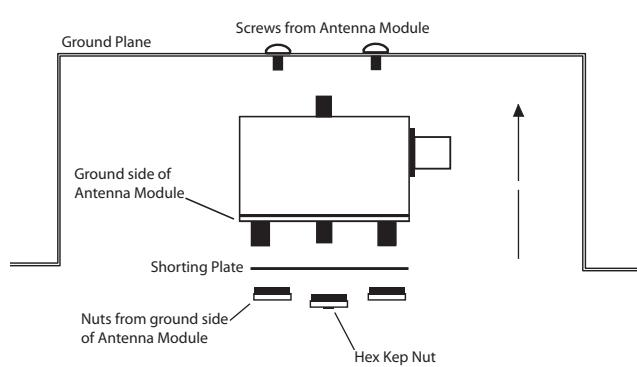
Diagram J. A reversed Antenna Module with Grounding Base and Shorting Plate.
