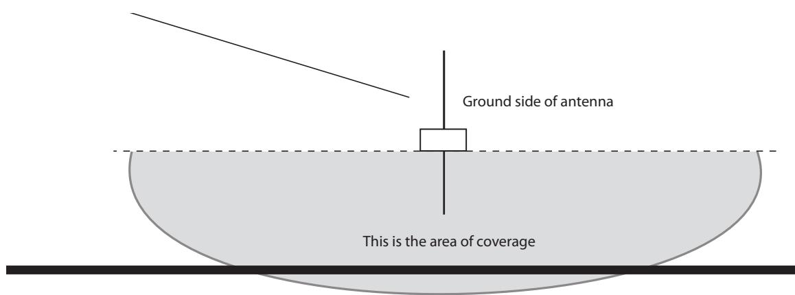
Diagram A. Antenna coverage patterns. In Scenario 1, the antenna is mounted low in the facility. The GROUND side of the antenna (marked on the module) should face down. In Scenario 2, the antenna is mounted high in the facility. The GROUND side of the antenna should face up.
