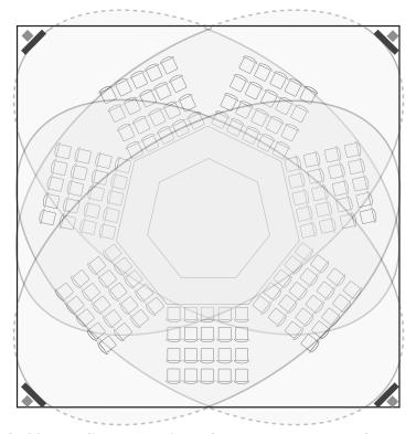
In this example a total of four radiators, one in each corner, ensures good coverage at all locations and orientations.
