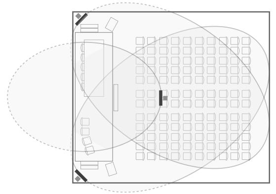
Except in small rooms, it is recommended that at least two radiators are used to prevent shading of the IR signal.
