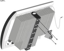
4 Pull CAT-5 and Coaxial cables through (if necessary)
