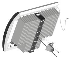
4 Pull CAT-5 and Coaxial cables through (if necessary)
