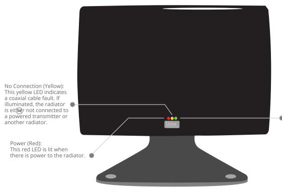
Carrier Present (Green): This green LED is lit when there is signal present to the radiator. During normal operation the red and green LEDs will be continuously lit (unless SW1 is off).
