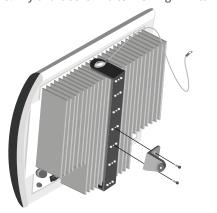
4 Pull CAT-5 and Coaxial cables through (if necessary)
