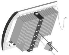
Pull CAT-5 and Coaxial cables through (if necessary)
