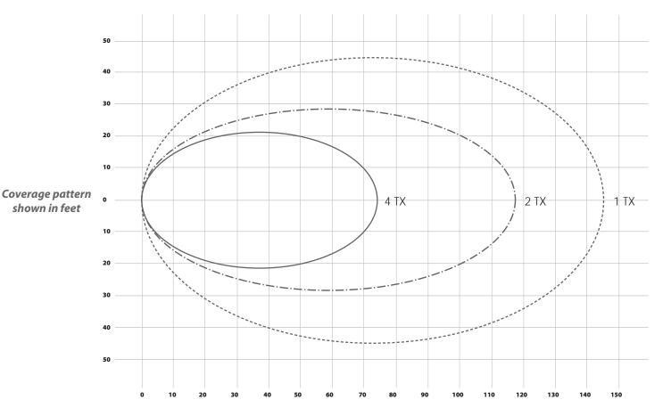
You should use the above coverage pattern to determine coverage of each radiator in your system, not by trial and error. The radiator will be stronger when new and therefore is under-rated by 40 percent and the coverage pattern above accounts for this. 40 percent degradation will occur after approximately 8,000 operating hours.
