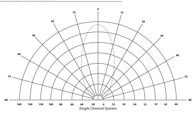
It is a good idea to provide over-lapping coverage (like in a sprinkling system) of the signal whenever possible to ensure that the signal does not have drop outs. In addition, you should provide special radiator coverage for shaded areas such as under a balcony or in the front of a room where the front mounted radiators do not provide enough coverage. The following diagrams illustrate these concepts.
