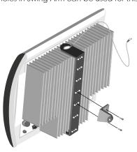
4 Pull CAT-5 and Coaxial cables through (if necessary)
